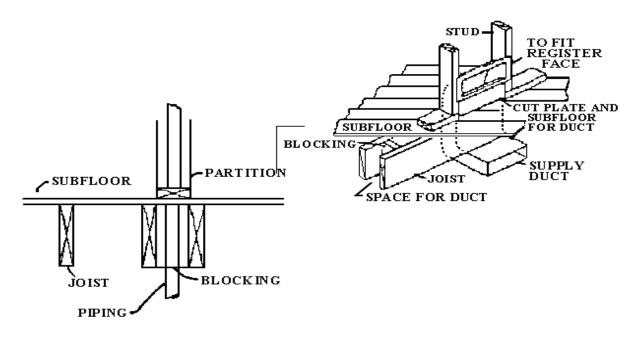
FLOOR FRAMING TO ACCOMMODATE PIPING AND DUCTWORK
