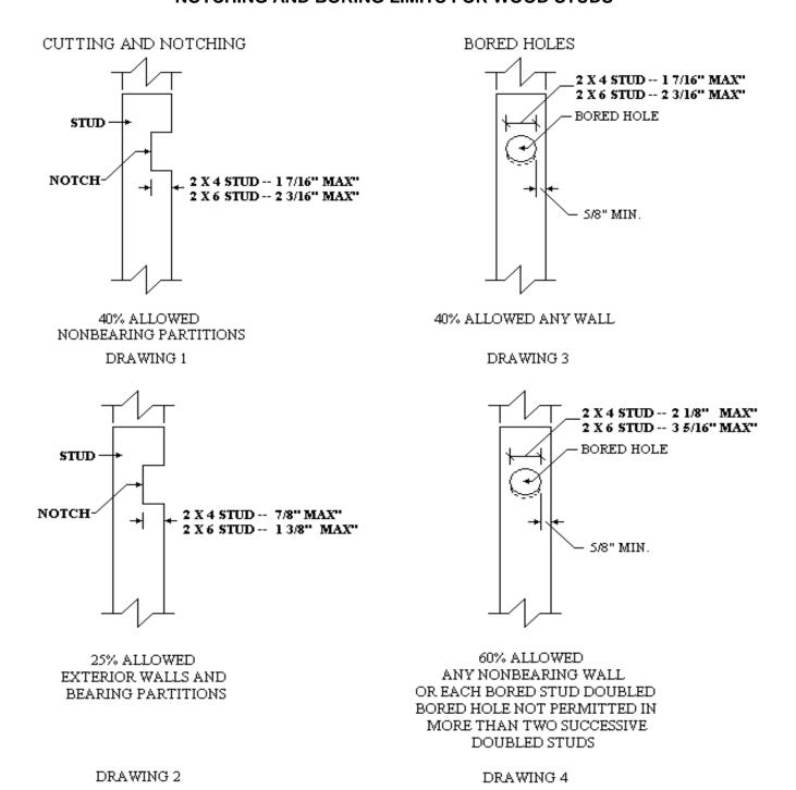
Figure 6: Maximum Allowed Notching and Boring for Typical Construction with 2x Studs
